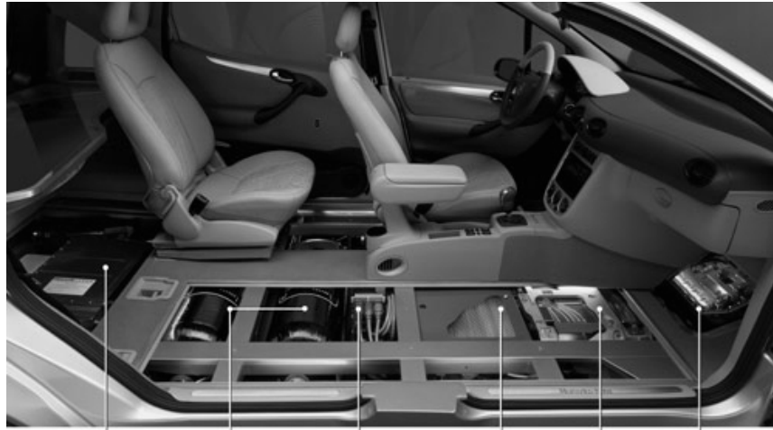
Battery Hydrogen Tanks Power Distribution Unit (PDU) Fuel Cell Module System Module Electric Motor
