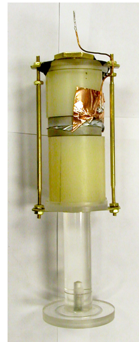
Figure D.12: Time-varying pressure applied by a weight hanging on a spring. (a) Signals from the electrodes; there is no intended phase relationship between the curves. (b) Photograph of the brace with plastic spacers and a copper electrode indium-bonded to glass.
