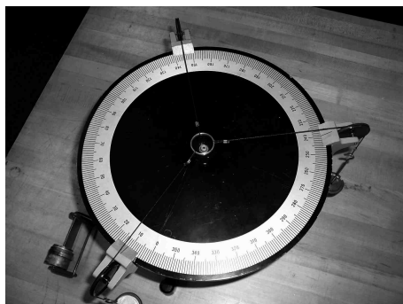
Figure 2: Top view of the force table
