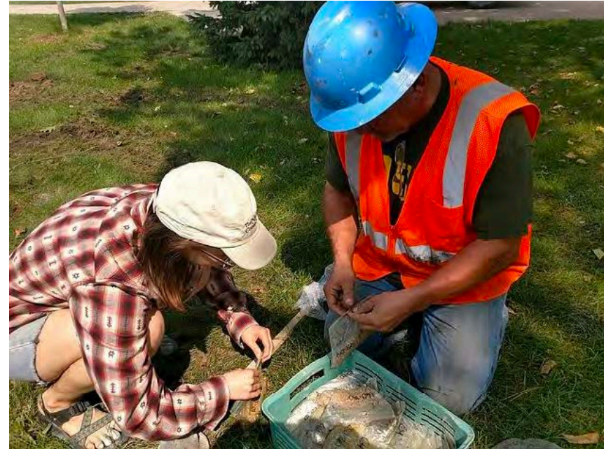
Carleton geology major and driller examining soil samples taken from a boring down to 520 ft. underground.
